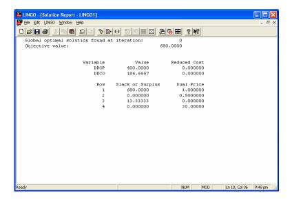
This window shows the values of each variable that will produce the optimal value of the objective function.
